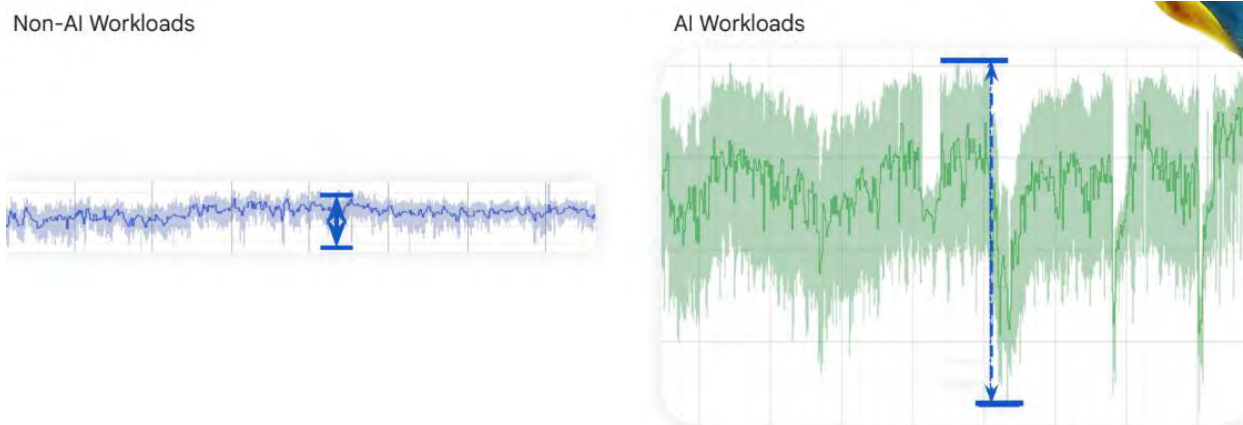
Figure 4: Computation power comparison between non-AI and AI workloads [45]. These plots, showing power consumption over time on an equal scale of magnitude, suggest a 15x difference in a peak-to-trough transition over a period of milliseconds.
