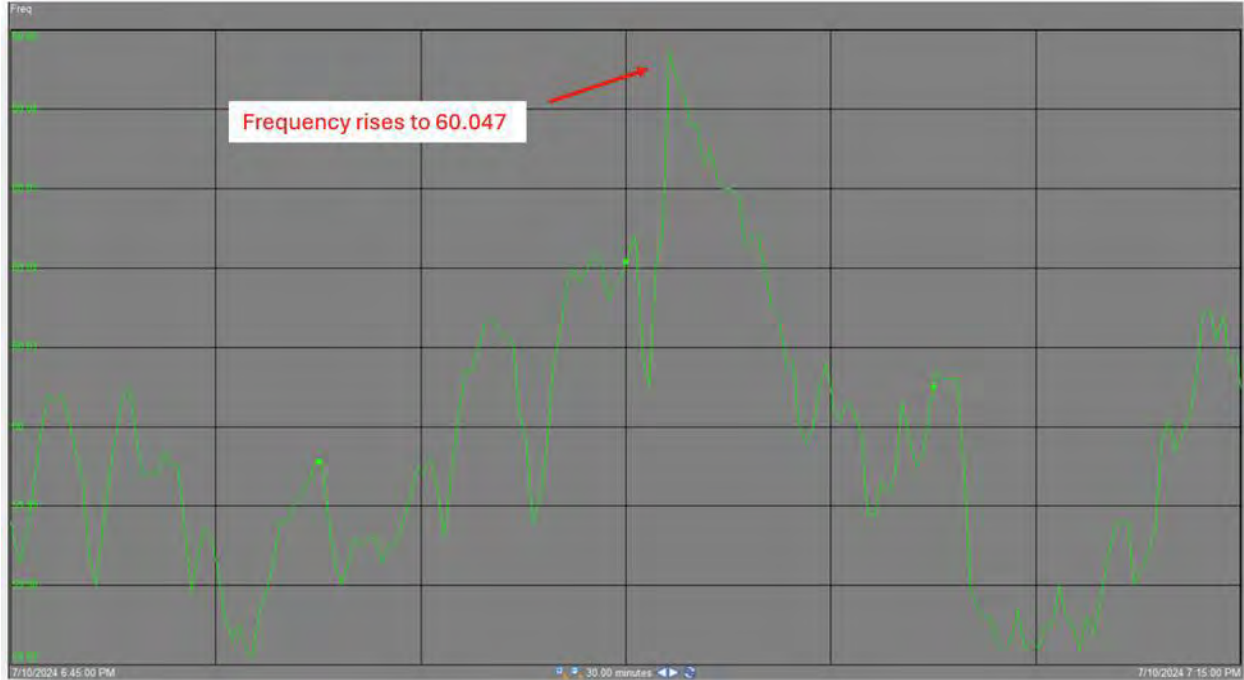
Figure 7: Frequency at time of large load loss in the same event [47].
